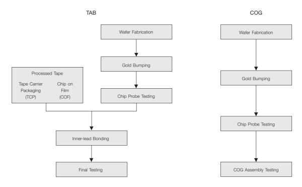
*Wafer Fabrication:* Based on our design, the foundry provides us with fabricated wafers. Each fabricated wafer contains many chips, each known as a die.
