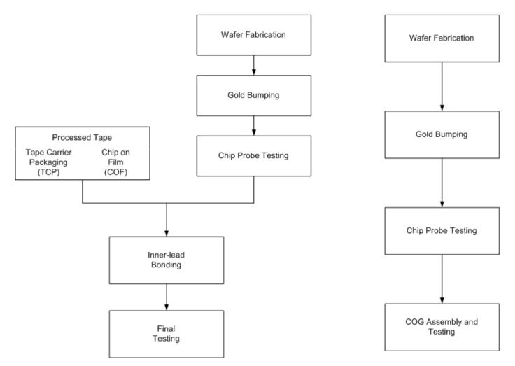
Wafer Fabrication: Based on our design, the foundry provides us with fabricated wafers. Each fabricated wafer contains many chips, each known as a die.
