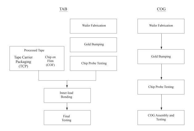
*Wafer Fabrication* : Based on our design, the foundry provides us with fabricated wafers. Each fabricated wafer contains many chips, each known as a die.
