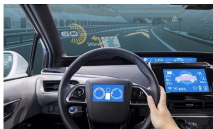
AR HUD (LCoS 2.0 Phase Modulation)
