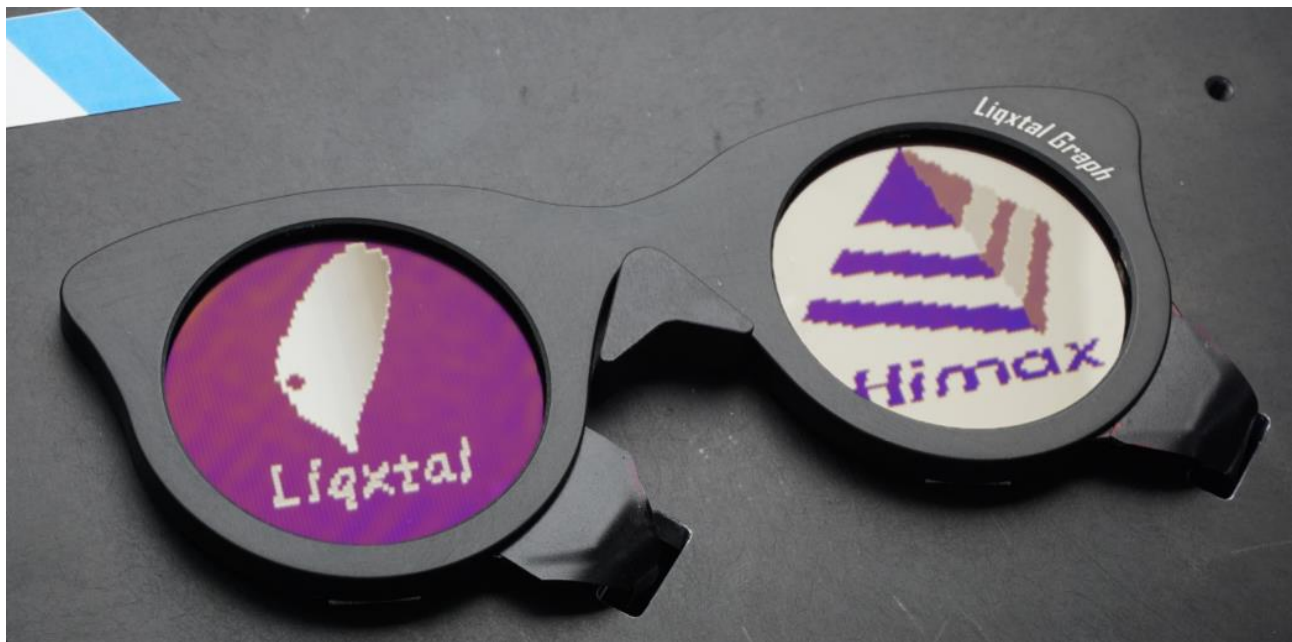
Liqxtal™ Graph Display Glasses: A patented technology with a design based on reflective TFT liquid crystal architecture that can display colored digital content, such as text, figure and animation, directly on the outer surface of the glasses lenses without compromising the user’s line of sight (Resources: Liqxtal Technology)
