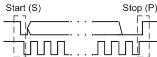
Figure 7.1: 2-Wire serial interface Start / Stop condition
