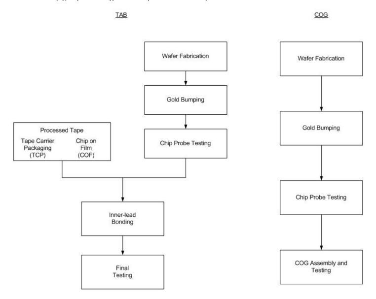
*Wafer Fabrication*: Based on our design, the foundry provides us with fabricated wafers. Each fabricated wafer contains many chips, each known as a die.
